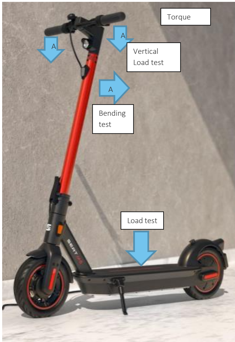
Fig. 4.1 Main e-kickscooter structural integrity tests of EN17128:2020
